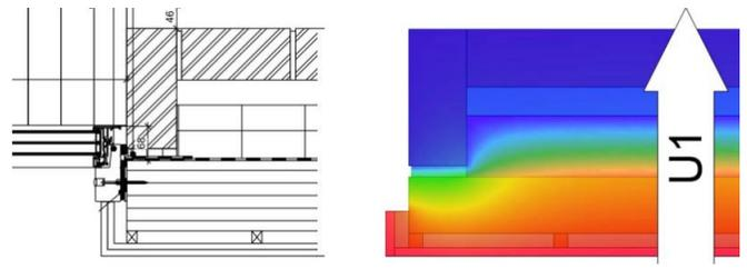
Improved Window Jamb detail including cavity closer: Architect's detail and thermal model
