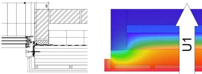
Window Jamb detail excluding cavity closer: Architect's detail and thermal model
