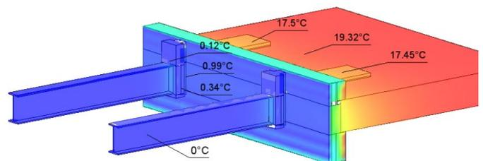
Steel balcony support structure penetrating wall insulation (thermal image)
