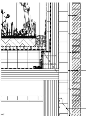
Wall and roof junction with structural timber (architect's detail and thermal image)
